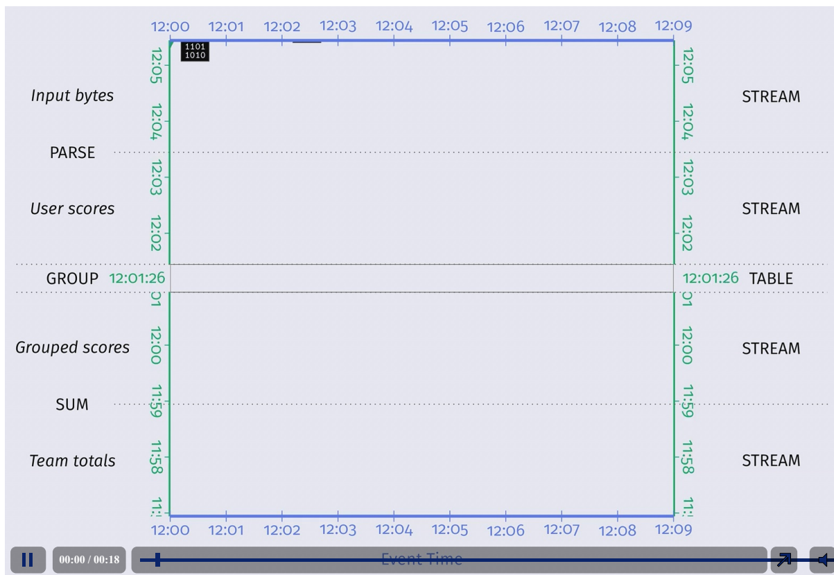
Figure 7-1. Summation via raw grouping of inputs with windowing and early/on-time/late triggering. The raw inputs are grouped together and stored in the table via the GroupByKey transformation. After being triggered, the MapElements lambda sums the raw inputs within a single pane together to yield per-team scores.
